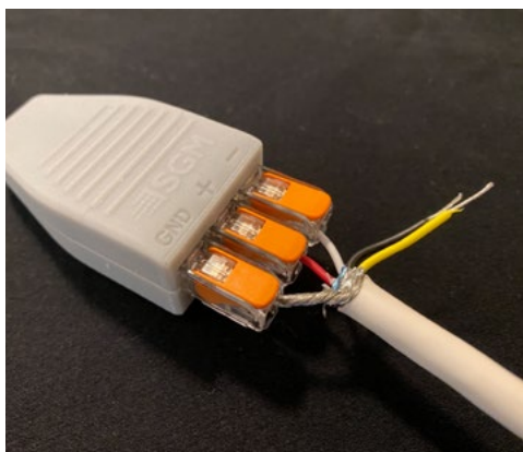
Figure 10: Connecting data to USB up-loader cable for POI fixtures
